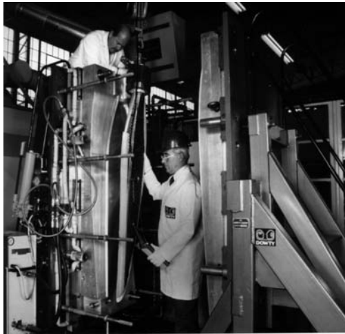
Figure 6.8. Preform and resin transfer mould.
