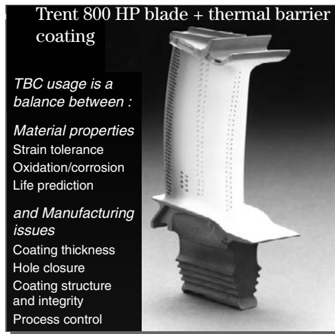
Figure 7.5. Trent 800 high pressure (HP) turbine blade, showing cooling holes and thermal barrier coating (TBC).
